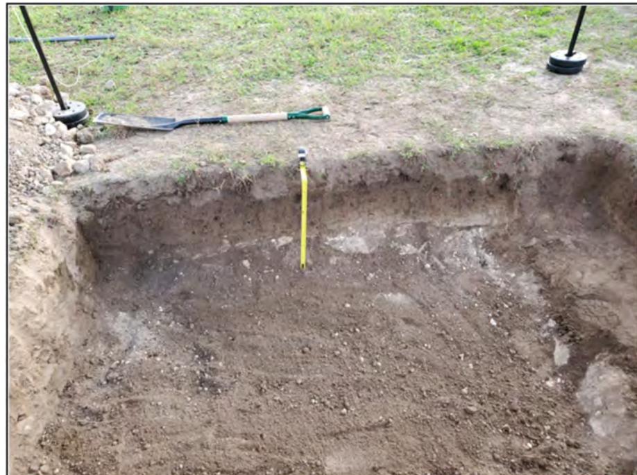
Figure 3-2. Hand-excavated pit at terminal depth.
