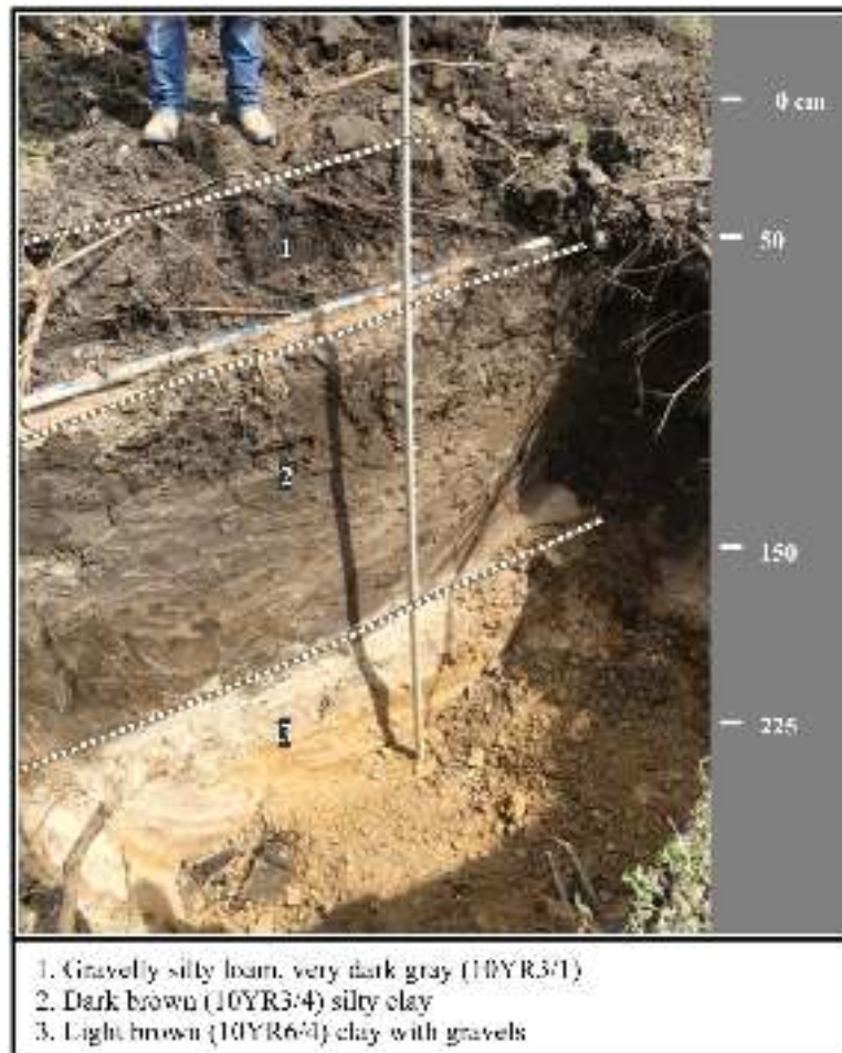
Figure 4-6. View of north wall profile for storm drain showing intact portion of the project area.
