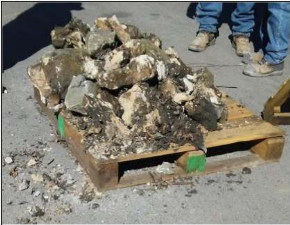
Figure 4-4. Limestone wall material removed from the canal and placed on wooden pallets.
