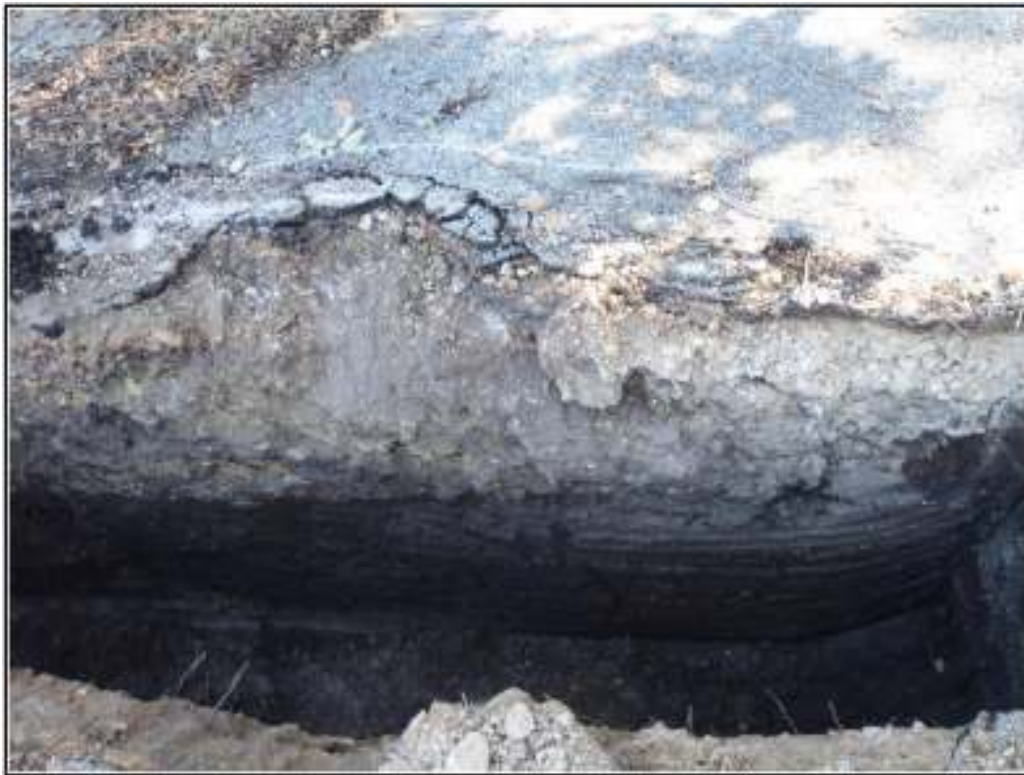
Figure 4-7. North wall of BHT 2, note dark gray clay zone under mottled gravel fill.
