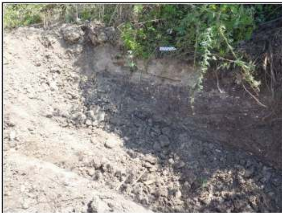
Figure 4-4. North wall of BHT 1 near western end of trench. Note the caliche layer that tops the clay loam mix.
