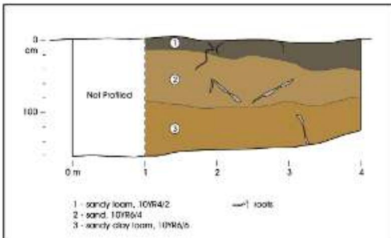
Figure 4-5. Backhoe Trench 2, west wall profile.
