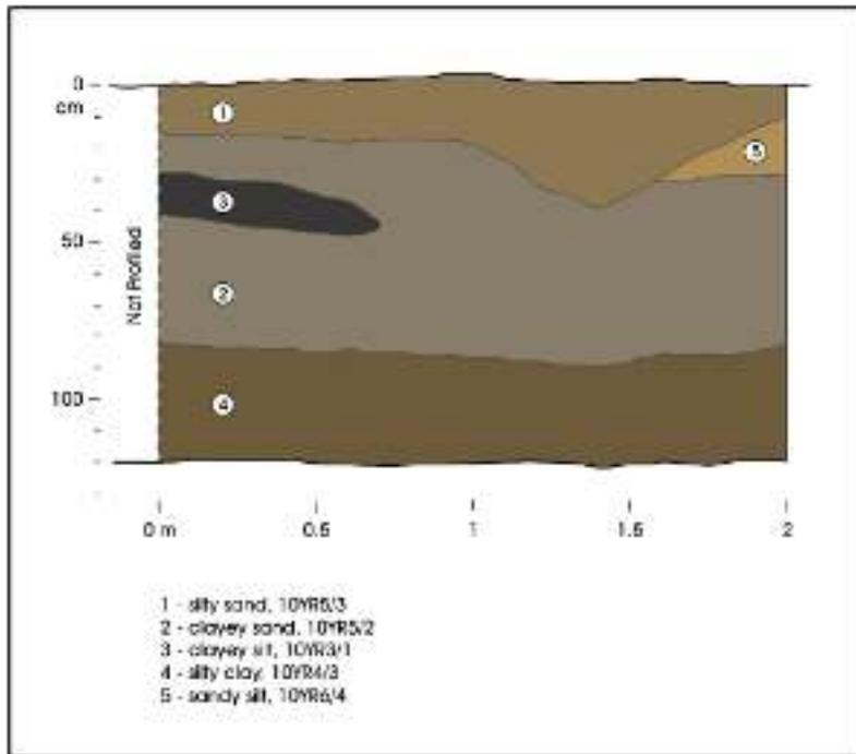
Figure 4-6. Backhoe Trench 3, east wall profile.
