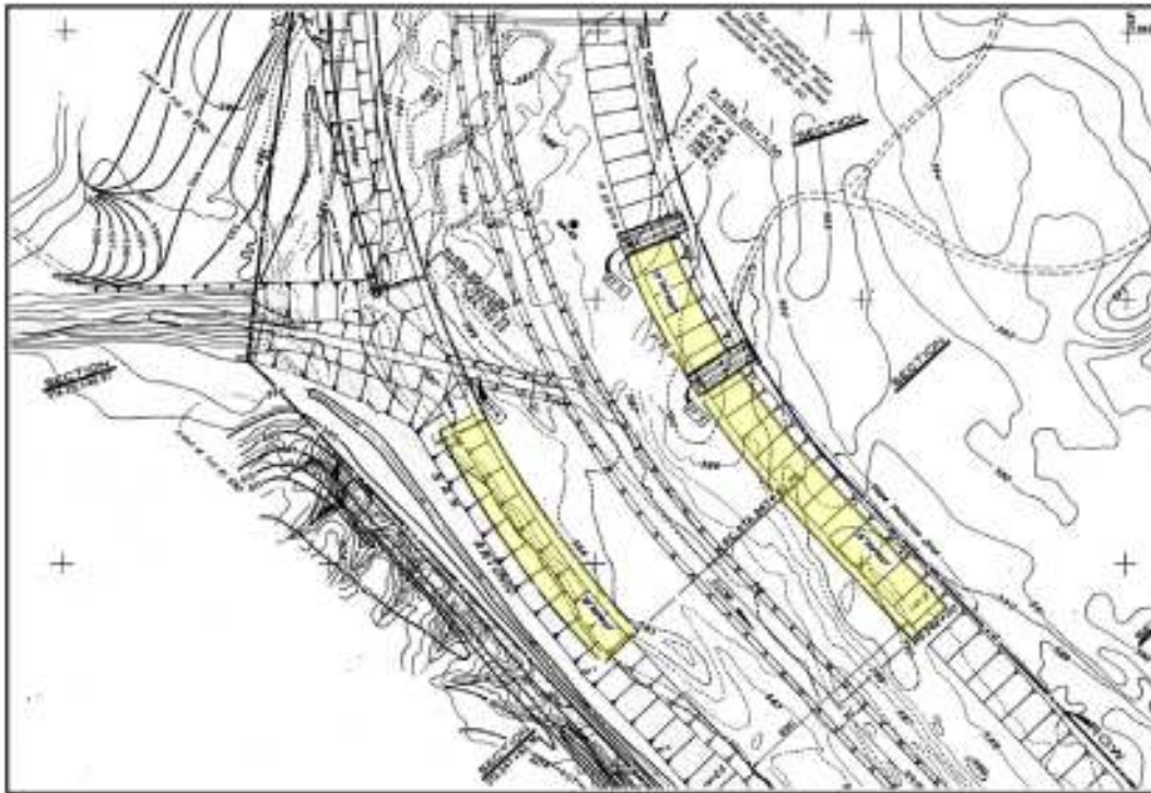
Figure 3-13. Detail plan for Area 3, from original plans for rechannelization of the river. Note reference to riprap along embankment walls (U.S. Army Corps of Engineers, Ft. Worth District, San Antonio River Channel Improvements Detail Plan, Sheet 27.2, 1957).
