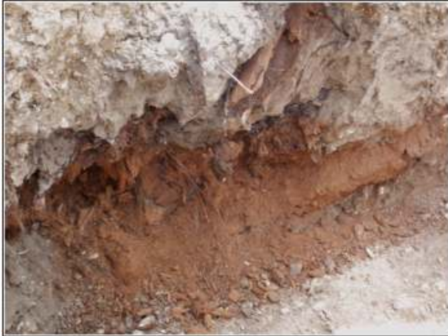
Figure 3-9. The west wall of Trench 4, showing several tree trunks buried in the fill at a depth of 3.8 m.
