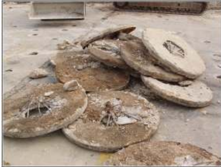
Figure 4-10. Wheels encased in concrete.
