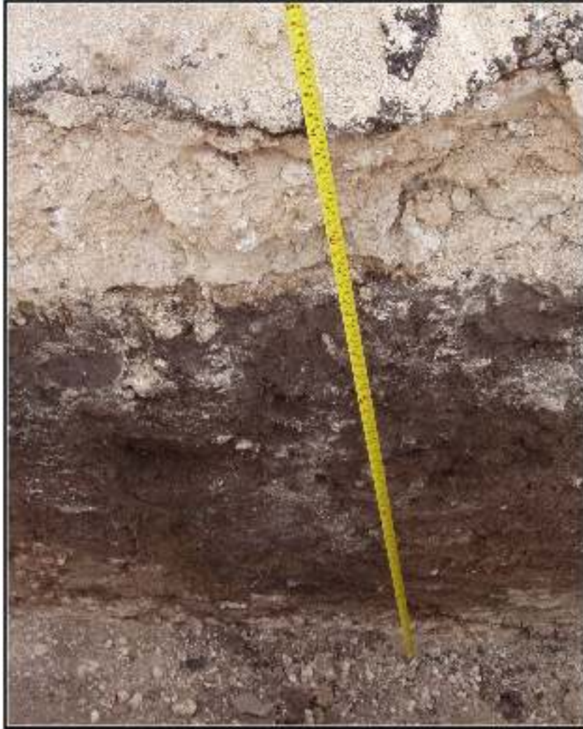
Figure 3-5. Photograph of the north wall of BHT #4, showing layers of modern fill.
