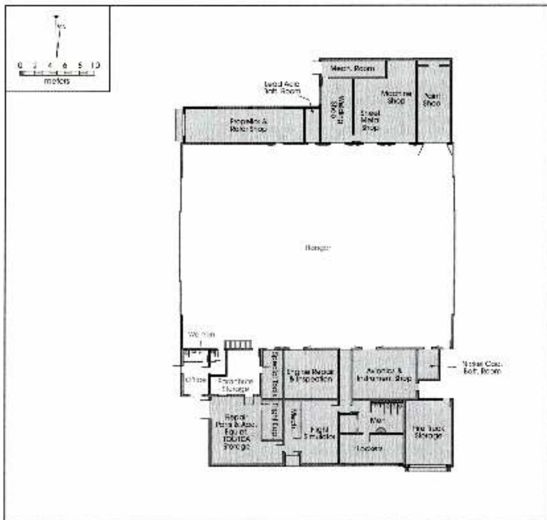
Figure 4-10. Floor plan of the 1975 addition to the Martindale AASF hangar shows additions made to the northern and southern faces of the hangar.
