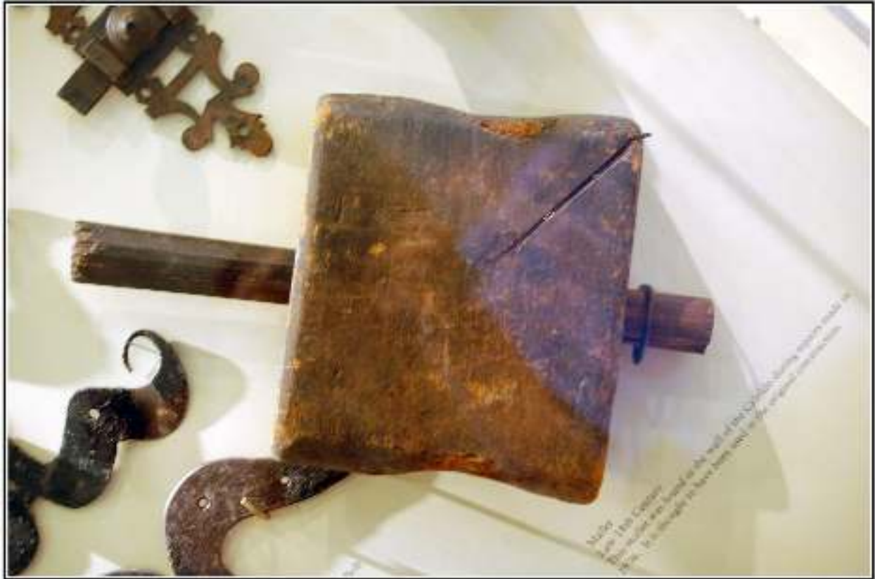
Figure 3-11. An eighteenth-century wood mallet, type used to pound a chisel, documented at The Cabildo.
