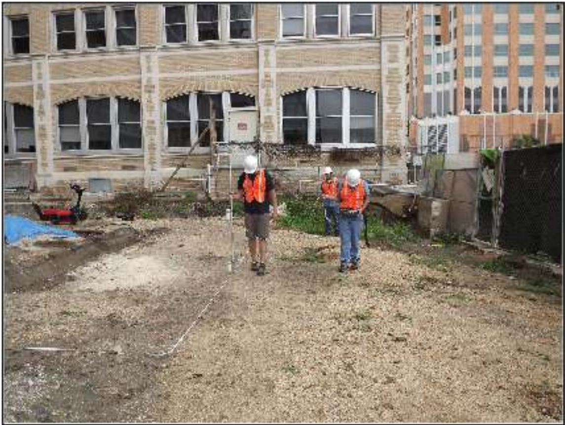
Figure 4-2. UTSA Geological Sciences Department conducting a magnetometer survey over a portion of the prayer garden.
