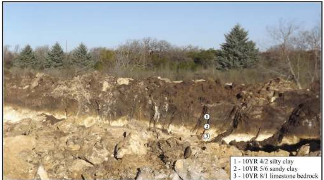
Figure 6-6. North wall profile of burrow pit within the central portion of the APE.
