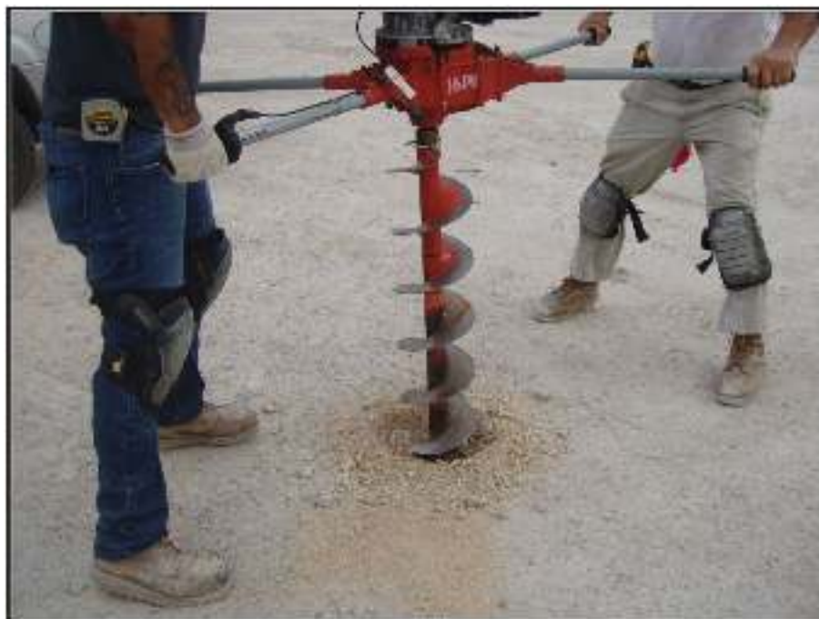
Figure 4-2. Gravel encountered in auger tests.
