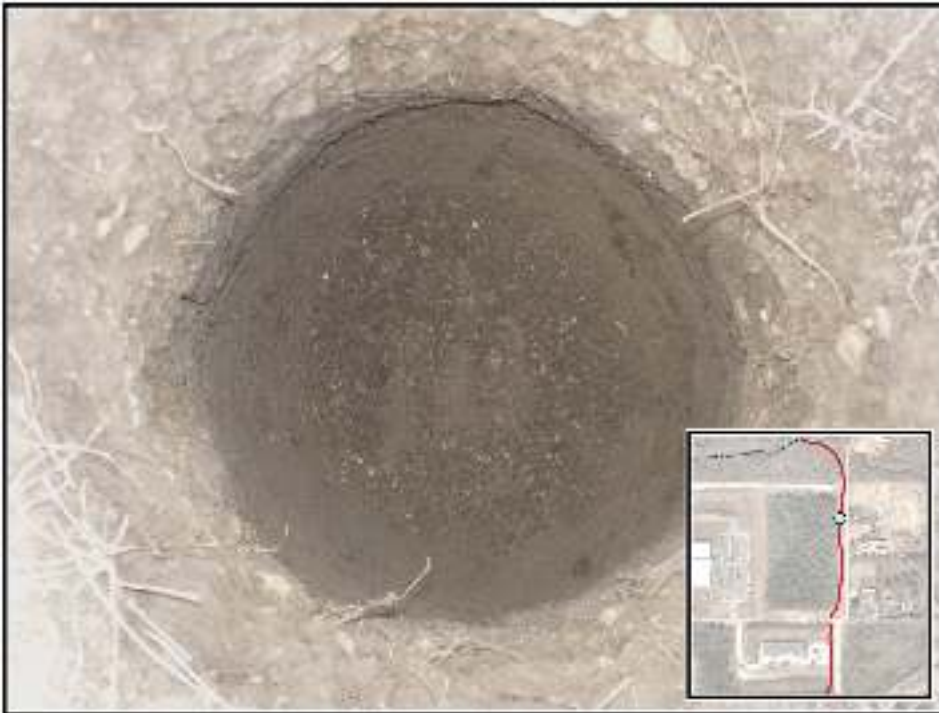
Figure 4-14. Photograph of ST 26 showing heavy gravel road base (blue dot on inset map represents approximate location of photographed area).
