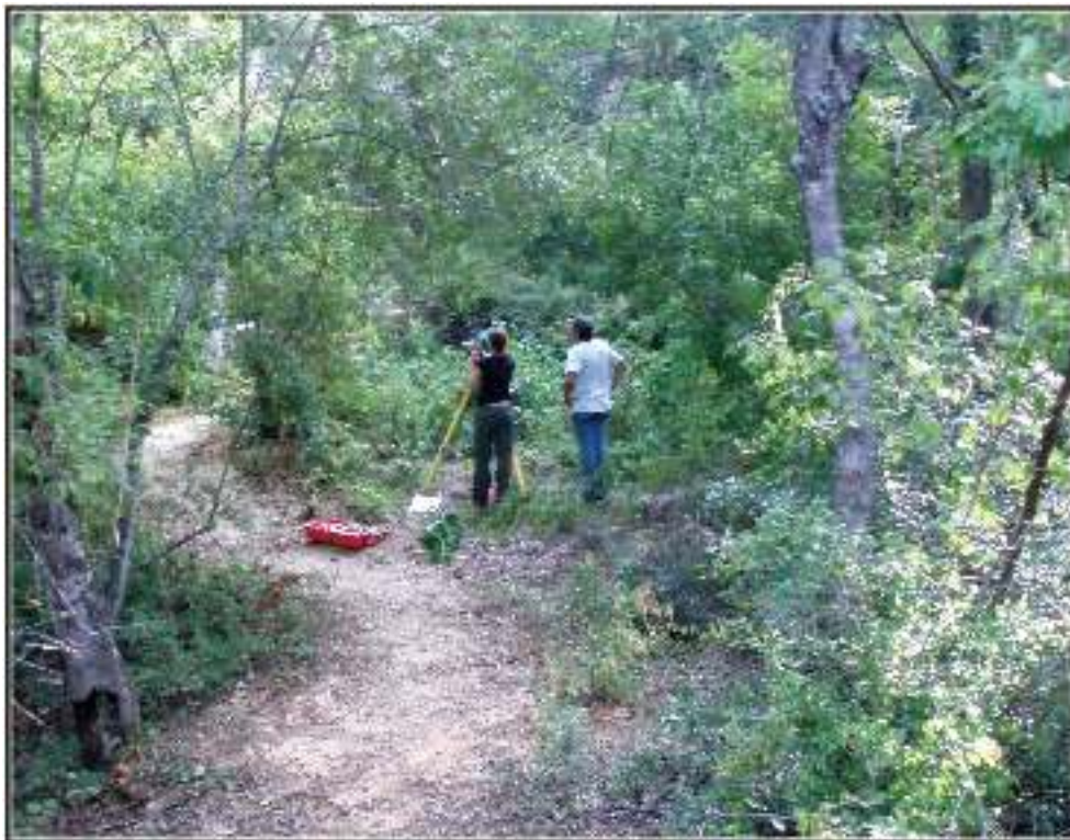
Figure 4-2. Use of a Sokkia total data station to lay test units on a magnetic north grid.
