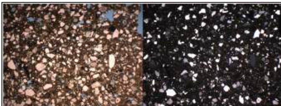
Figure 8-11. Very sandy-sand tempered sample (SAAN-32605-37) at 4x magnification in plane light (left) and cross-polar light (right).
