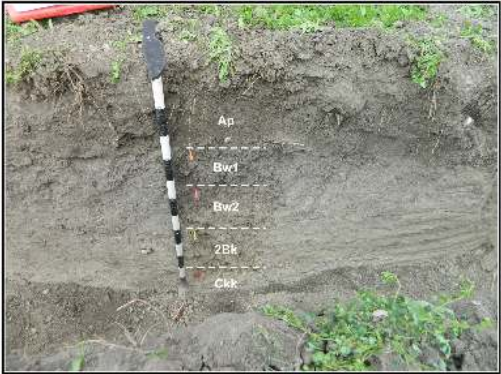
Figure 5-6. BHT 3 soil profile. An erosional unconformity exists between the Bw2 and 2Bk horizons.
