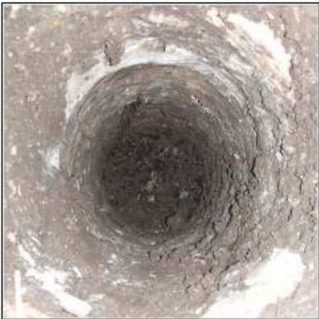
Figure 5-18. Auger Boring 1, note limestone zone near top of unit identical to Zone 2 in BHT 9 profile.
