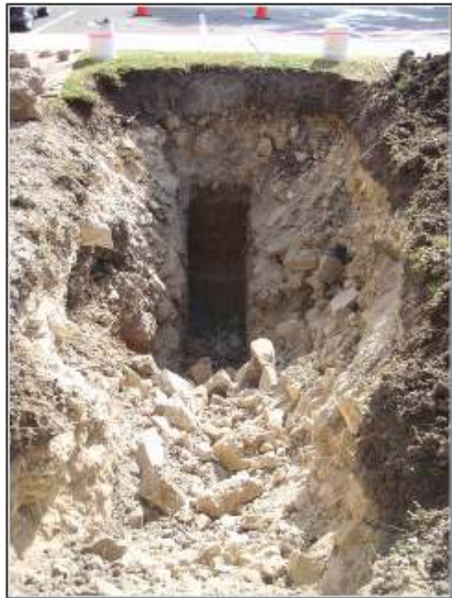
Figure 5-4. Eastern end of BHT 2 showing massive zone of unconsolidated fill materials overlying a deeply buried clay deposit. View is looking east.
