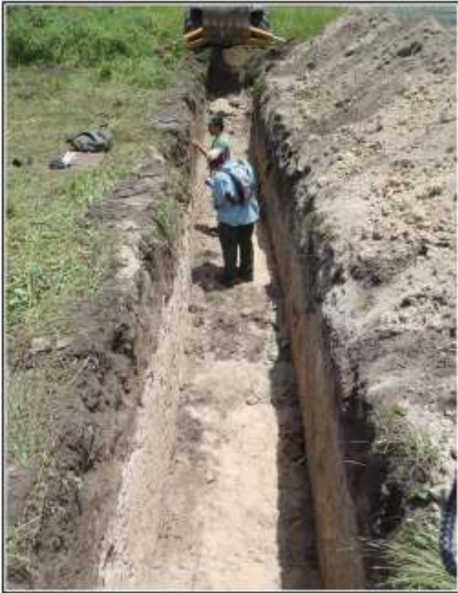
Figure 5-29. Profiling of BHT 27 showing distinct change between upper dark soils and caliche.
