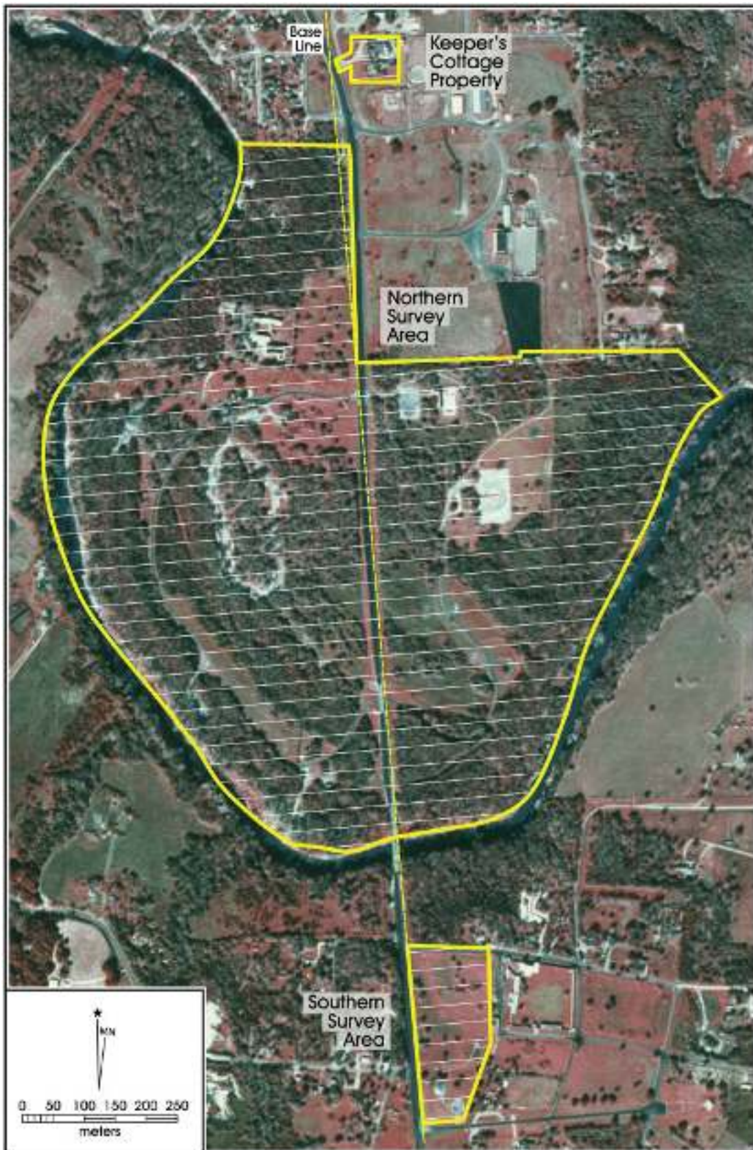
Figure 4-1. Aerial photograph showing the project area with survey transects set at 30 meter intervals.
