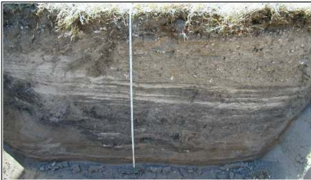
Figure 5-11. Photographs of Beaumont Ridge zone at 33+689, showing large, naturally refilled erosional channel. Note shell at bottom of erosional channel and modern fill above the natural laminated sand and clay fill.
