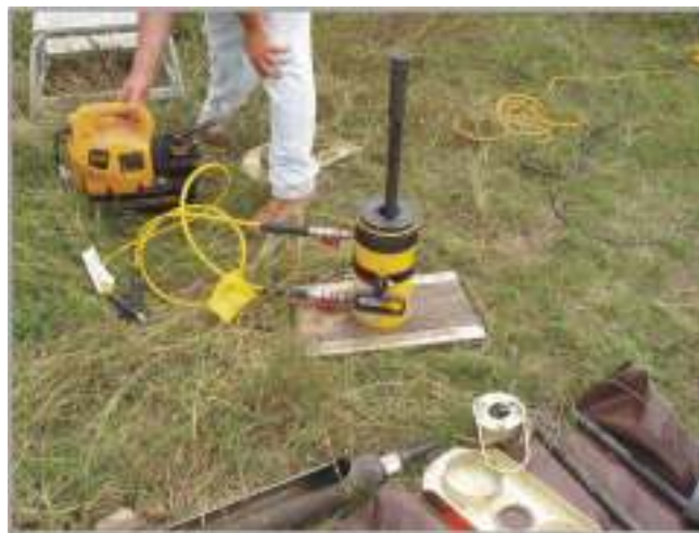
Figure 4-4. Hydraulic lift being used to extract the gouge from Core #2.
