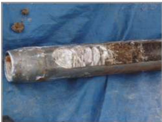
Figure 4-3. Limestone fill encountered at the bottom of Core #1.
