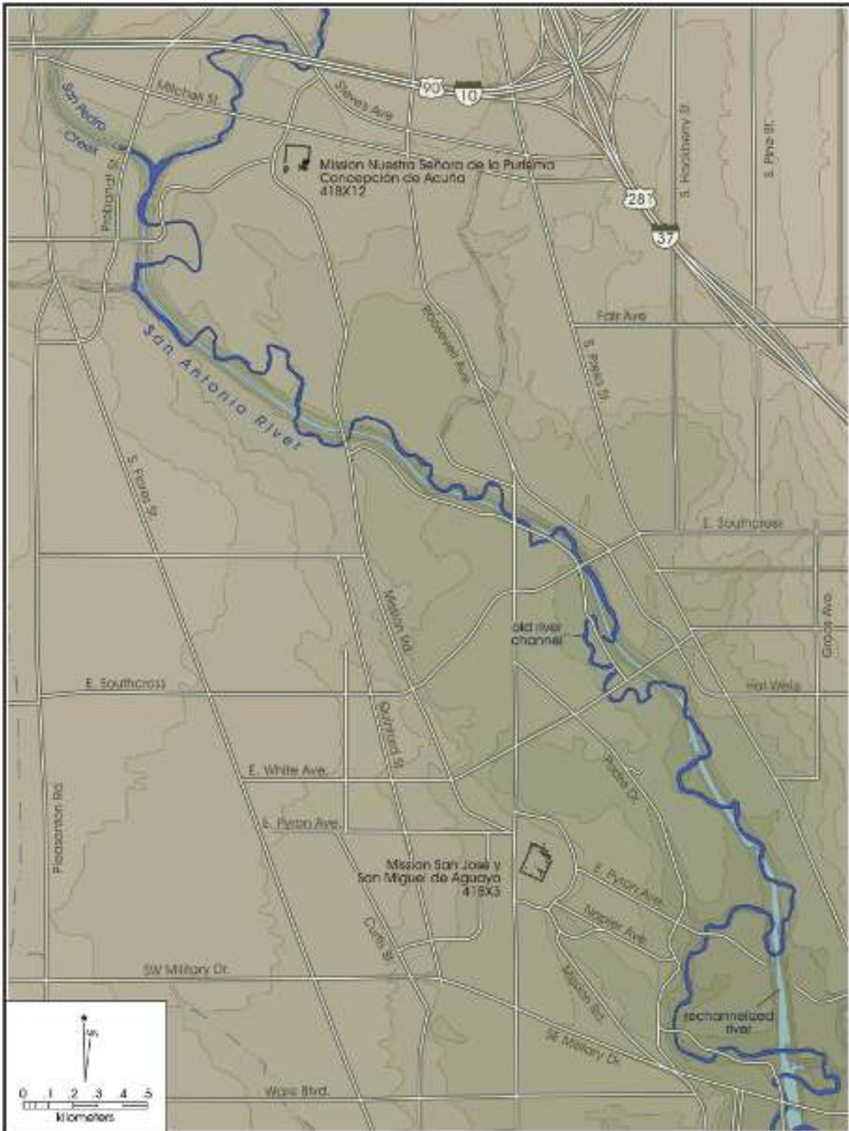
Figure 1-2. The portion of the San Antonio River in the Mission Trails Enhancement Project, Package 2 and 3 area, showing the old river channel and the rechannelized river.
