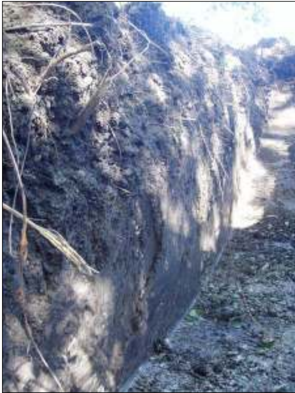
Figure 16. Photograph of Backhoe Trench 3 showing 1.25 meters of silty clay.
