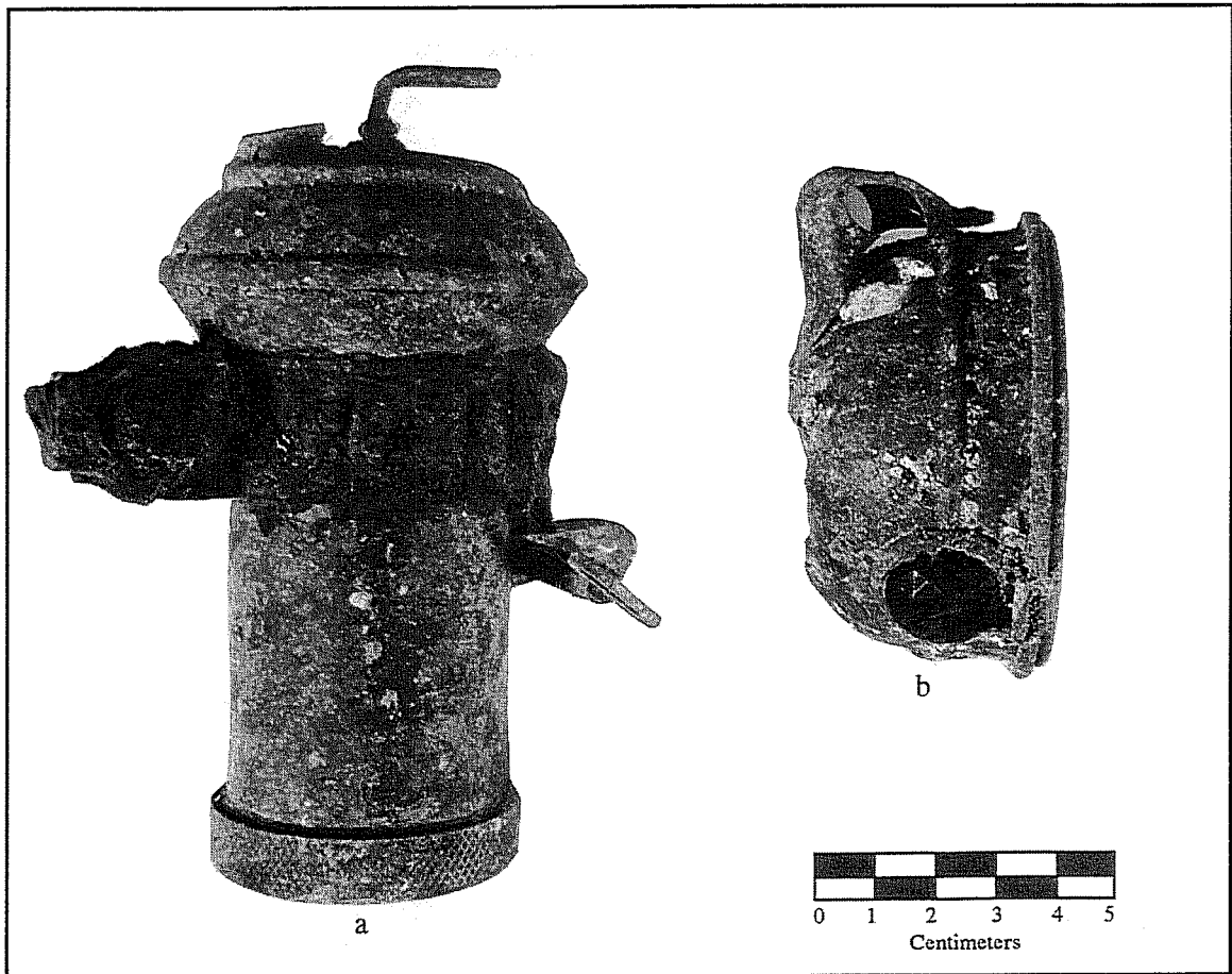
Figure 19. Carbide bicycle lamp . a. main portion; b. reflector.
